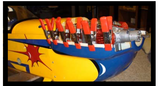
Rebuilding the cowling after cutting the top off
